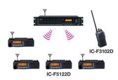
The IC-F5122D series allows you to call individual or group users. The radio automatically sends own ID number when the PTT button is held down. The alias name or individual/group ID is displayed on the LCD while receiving a message allowing you to identify who is calling.
