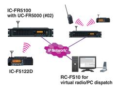
When using the IC-F5122D series in IDAS multi-site conventional mode, the IC-F5122D can communicate with other IDAS radio users working with other repeater sites and/or virtual radio/PC dispatch stations on the IDAS network.
