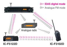
The IC-F5122D series can receive both analogue and digital mode signals on a single channel and automatically selects the received mode to reply to the received call, while the talk back timer remains. It's a smart way to grow into digital radio – at your own pace, as your budget and comfort allow.
