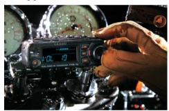
Enjoy your FTM-10R/E\* outdoor with your motorcycle, SUV or RV anywhere! The commercial grade front panel meets the IP57 standard. (Waterproof at 3 feet (1 m) for 30 minutes, and protection against dust.) All connectors are waterproof.
