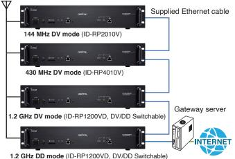
Up to 4 modules can be connected to one gateway server. The DD mode repeater must be directly connected to the gateway server.
